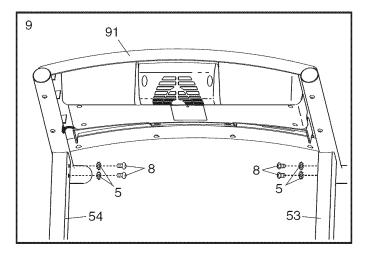
10. Start two M8 x 15mm Bolts (8) with two M8 Star Washers (5) into the Uprights (53, 54). **Then, firmly tighten all six M8 x 15mm Bolts (see step 9).**
